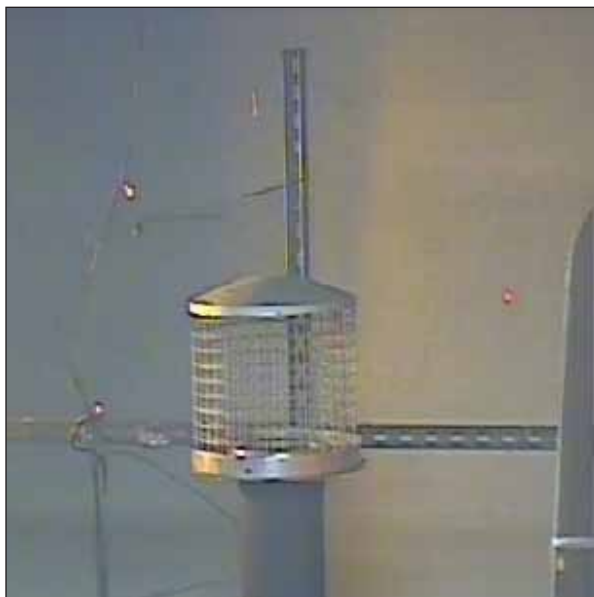
Figure 48a, b. Capped coarse mesh spark arrestor.
