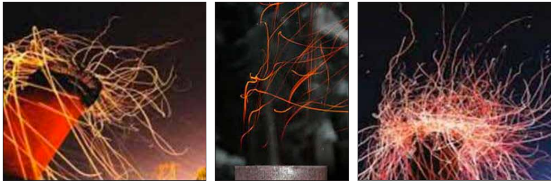
Figures 5-7. Direct spark ignition of thatch.
